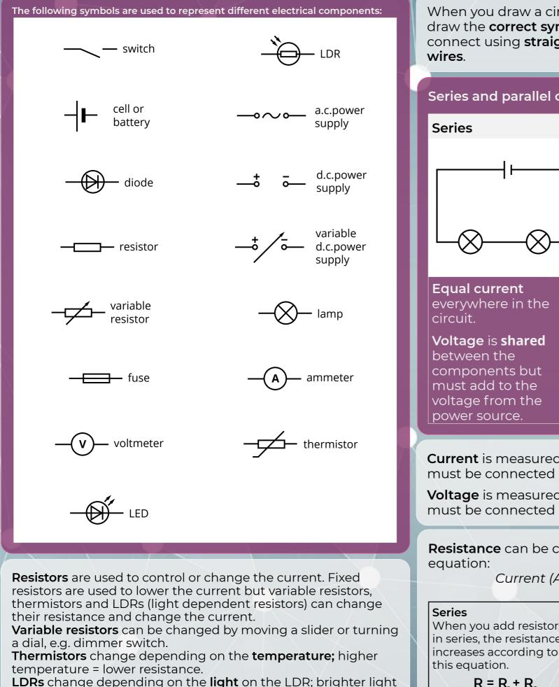
When you draw a circuit; remember to draw the correct symbols in place first then connect using straight lines to represent the
